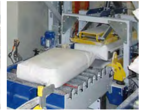
Bag conditioning by top flattening and vibrating
