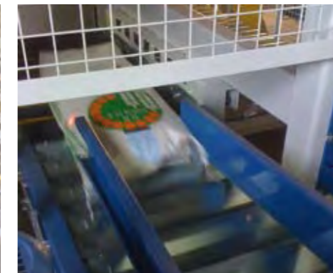
Bags conditioning by motorised squared rollers
