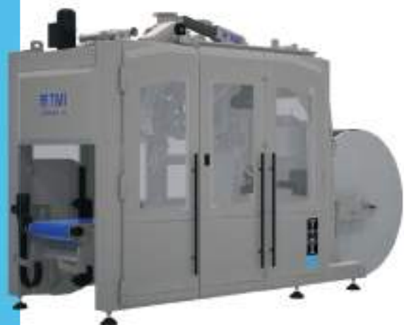
Hygienic horizontal FFS bagging machine for plastic bags from tubular film.
